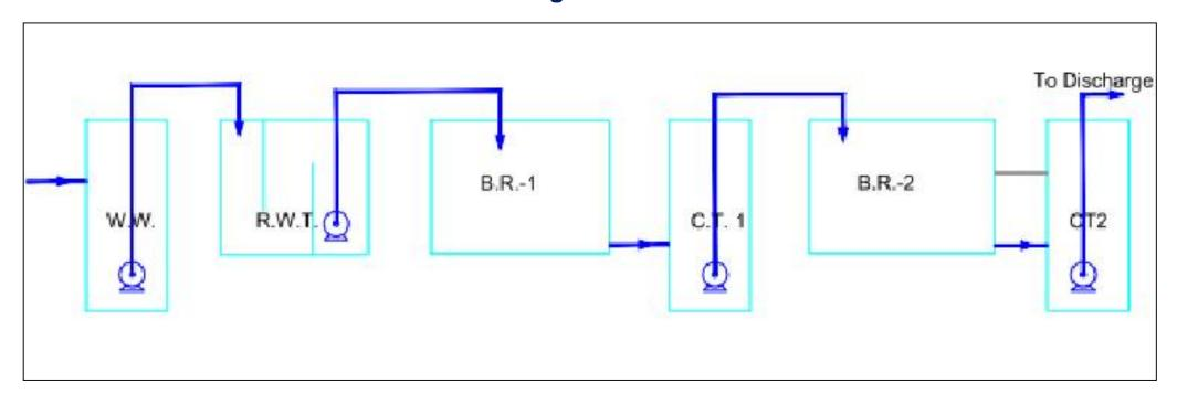
Raw sewage is collected in Raw Water Tank (RWT) after initial screening and settling. The raw sewage is pumped on the top of a SBT Bio Reactor where it percolates through a geological media. The treated water from BR-1 is collected and again treated to attain reuse quality and then collected at the bottom of the Bio-Reactor (BR-2) and stored in a Treated Water Tank (TWT).
